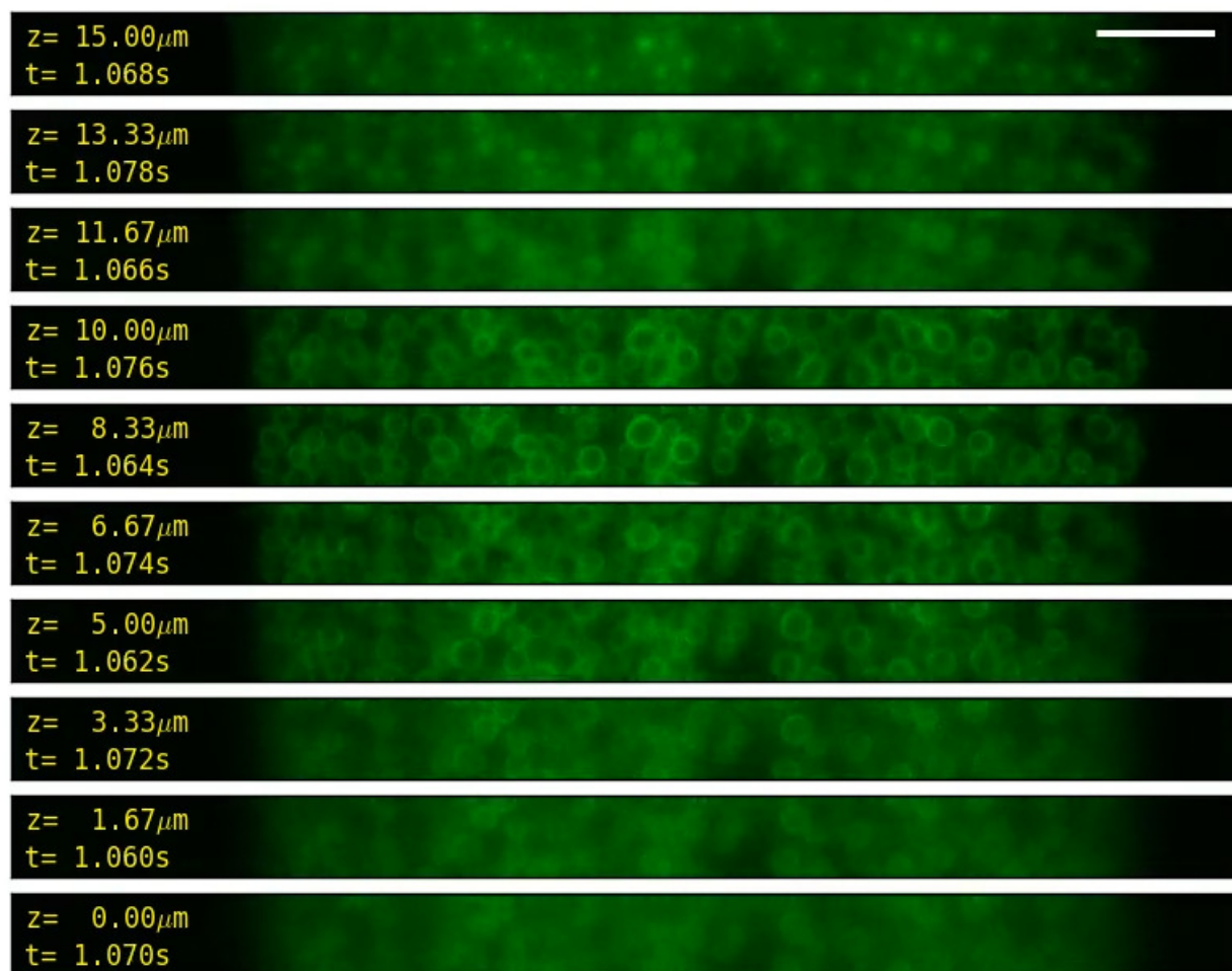
Figure 2: Remote refocus enabling fluorescent imaging of yeast at 50 volumes per second. Yeast flow through a microfluidic channel 150 \mu\text{m} wide by 10 \mu\text{m} deep. Volumes consist of 10 z-slices at 1.66 \mu\text{m} intervals, with bi-directional scanning and 2 ms exposure time per 2D image. The image is cropped to give a 207x14 \mu\text{m}^2 field of view, each slice of each volume is displayed simultaneously, and the scale bar is 20 \mu\text{m} .
