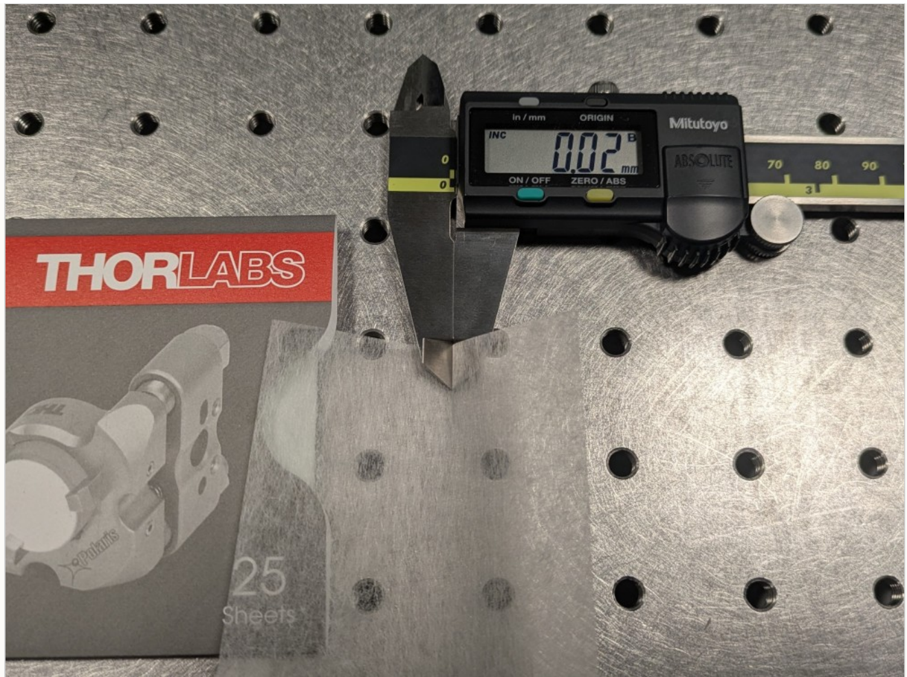
Figure A6: Thorlabs lens tissue MC-5 thickness. Here we show the measured thickness of Thorlabs lens tissue (MC-5) at about 20–30 \mu\text{m} . With the calipers adjusted to 20 \mu\text{m} the tissue is pinched in place, at 30 \mu\text{m} it will slide out.
