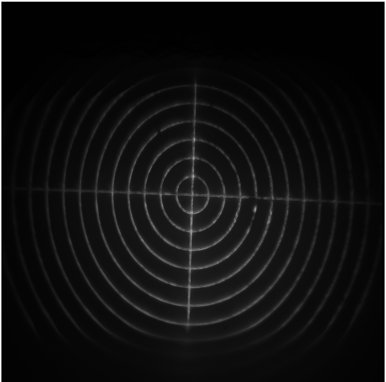
Figure 8: Target image stack using the AMS-AGY v1.0 objective with a 30° tilt. This \sim 240 \times 240 \mu\text{m}^2 image shows a maximum-intensity Z-projection of a tilted image stack of the remote field of view. The illumination shows interference patterns from the coherent 488 nm excitation and is slightly off-centre (as seen in the saturated image). Note that without any transformation, the raw projection shows the target 'stretched' along the Y-axis due to the tilt of the objective. Re-scaling this axis by y \cos(\alpha) ( = 0.866 for 30^\circ ) restores the image to its correct scale (where \alpha is the tilt angle). Again, the saturated image shows the ground glass edge of the AMS-AGY v1.0 objective (as designed). For data processing see the readme.txt .
