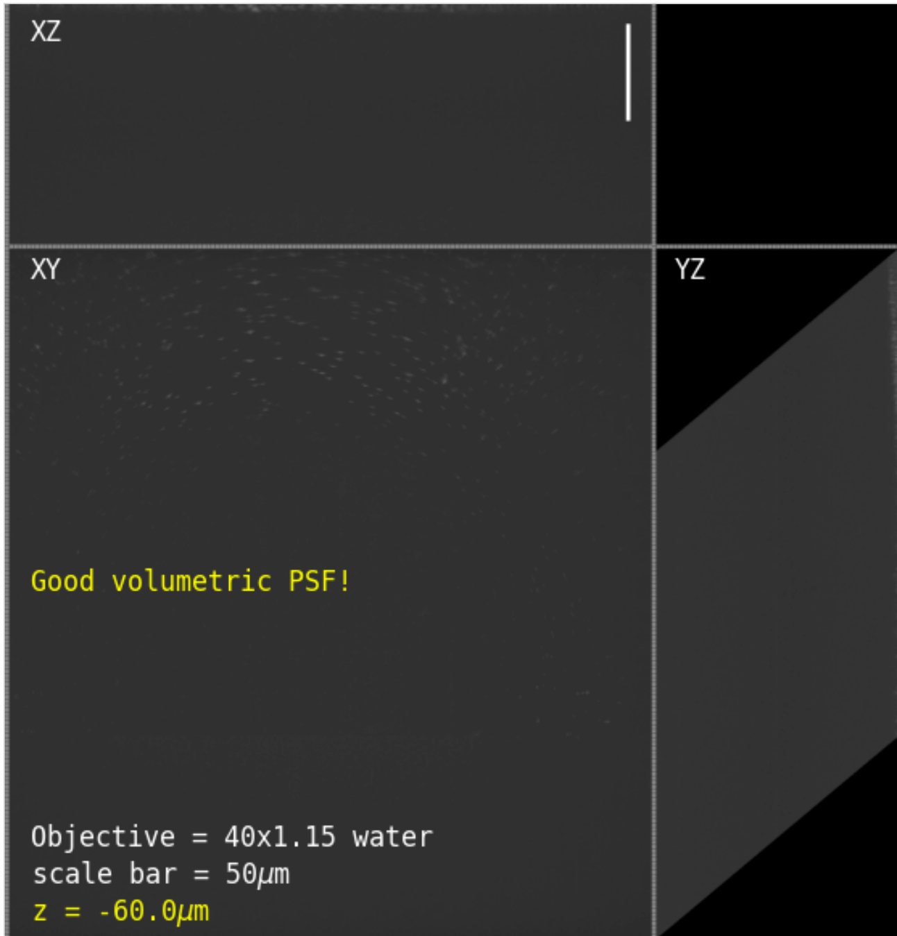
Figure 8: PSF vs standard focus for a 40x1.15 water objective. This animation shows the volumetric point spread function of a Nikon 40x1.15 water immersion objective as a function of standard focus ( z ). The fluorescent beads were prepared in a watery gel according to this protocol . Since the sample RI matches the water immersion the PSF is insensitive to standard focus, allowing an increased depth of focus (standard focus + RR) when using the microscope in this modality. Note: each frame of the animation shows the max projections of the entire volume ( \sim 330 \times 355 \times 125 \mu\text{m}^3 ) in traditional XY, XZ and YZ coordinates.
