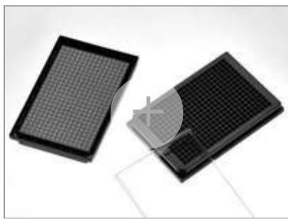
384 well glass bottom plate. Black polystyrene frame with high performance #1.5 cover glass (0.170±0.005mm), with lid, Individually packed. Designed for high resolution imaging such as confocal microscopy.
