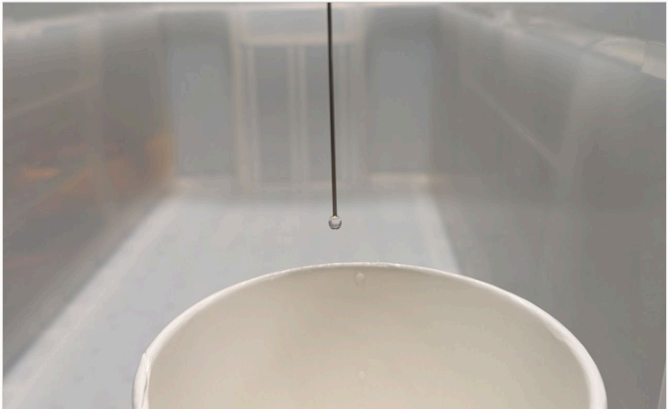
Figure A7: retained droplet. Here's an example of a retained droplet from early testing with a small diameter stainless steel tube (a 2 inch long version of the ~1.7 mm holding tube ). We found that this configuration would retain a ~50 \mu\text{l} droplet which was way too large for the target dispense range of 10 \mu\text{l} to 100 \mu\text{l} .
